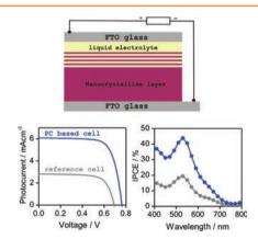
Highly efficient, thin, dye-sensitized solar cells can be designed through the integration of 1D photonic structures of optimized porosity, with increases in both the device photocurrent and the photovoltage. Devices with enhanced efficiency are obtained while preserving the transparency, which is a topic of major interest due to possible applications in building integrated photovoltaics (BIPV).
