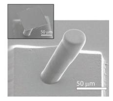
Gecko-inspired angled elastomer micropillars with flat or round tip endings are presented as compliant pick-and-place micromanipulators. The pillars are 35  $\mu$ m in diameter, 90  $\mu$ m tall, and angled at an inclination of 20°. Through shear displacement control, pick-to-release attachment force ratios of 39 to 1 are achieved and micromanipulation is demonstrated.
