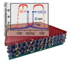
Organic spin valves show many promising features but remain poorly understood. An experimental study of  $C_{60}$ -based spin valves is presented and their behavior is modeled with spin-polarized tunneling via multiple intermediate states. Analogous to the conductivity mismatch in the diffusive regime, the magnetoresistance decreases with the number of intermediate tunnel steps, regardless of the value of the spin lifetime.
