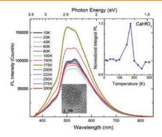
Optical properties of SrHfO<sub>3</sub> and CaHfO<sub>3</sub> nanoparticles with sizes as small as 1.6 nm are reported. An unexpected and strong luminescence from the undoped nanoparticles is observed in the visible spectrum over a wide temperature range, also exhibiting sensitivity to temperature variation and surrounding ambient (vacuum/air) as well as exposure time to UV light.
