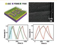
Microelectrodes of an all-solid-state flexible micro-supercapacitor are prepared using in situ electrodeposition of polyaniline nanorods onto the surface of reduced graphene oxide patterns. The micro-supercapacitor possesses high electrochemical capacitance and good stability.
