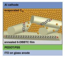
Self assembly can be exploited to engineer the interface and morphology between the single crystal cables of donor material (6-DBTTC) and polycrystalline acceptor ( $C_{60}$ ) to create an interpenetrating network of pure phases expected to be optimal for photovoltaic device performance. These strategies facilitate 3D nanostructured photovoltaic cells made with the simplicity and control of bilayer device fabrication.
