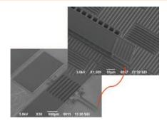
The advanced fabrication of silicon microstructures of various shapes and silicon microsystems of high complexity using electrochemical micromachining (ECM) technology is described. ECM technology makes use of a dynamic control of the electrochemical etching anisotropy, which allows silicon dissolution to be switched in real-time from the anisotropic to the isotropic regime, to enable the low-cost fabrication of microstructures and microsystems using both functional and sacrificial structures.
