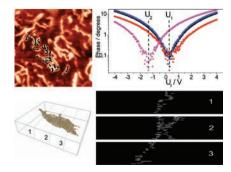
The conductive graphene network in a conductive graphene/polystyrene composite sample is separated from electrically isolated graphene sheets by analyzing the same area with conductive atomic force microscopy (C-AFM) and electrostatic force microscopy (EFM). The novel technique based on combination of a scanning probe microscope and microtome is utilized for 3D reconstruction of the graphene sheets in the polymer matrix with z-resolution in the order of  $\approx$  10 nm.
