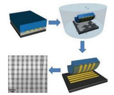
Metal electrode crossbar arrays with feature sizes in the nanometer range are fabricated by combining nanoimprint lithography with a universal and gentle printing method. The feasibility of this process is demonstrated by assembling 8 bit  $\times$  8 bit crossbar arrays. Metalmolecule metal junctions are realized and electrically characterized by incorporating two types of conductive polymers into the crossbar structures.
